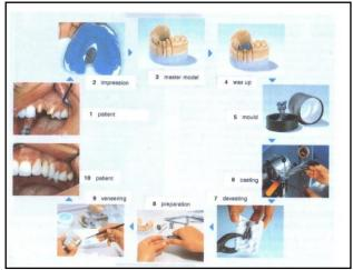
Fig. 5: Lost-wax casting method
